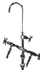
LS - WT. 4a 3-way water tap having swain neck in the centre and 2 side straight type taps
