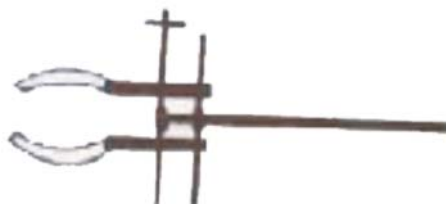
LS - RCL. 4/B RETORT CLAMP ( GIANT SIZE) of bigger & stronger jaws of C.I. to grip upto 200 mm dia
