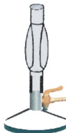
LS-FB 1 FISHER TYPE Burner with stop cock giving long wide strong flame.
