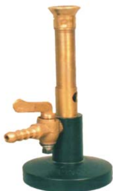
LS-BB1 BUNSEN BURNER giving long narrow pointed flame
